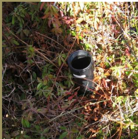
Piezometer well, with its cap removed for a water sample, being used to measure water quality and quantity
